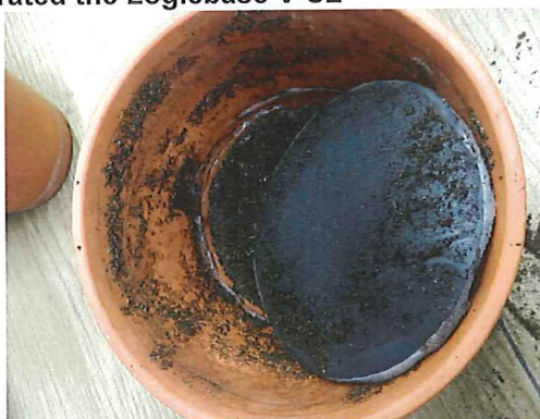
Photo No. 4 and 5 – The roots have not penetrated the Logicbase V-SL
