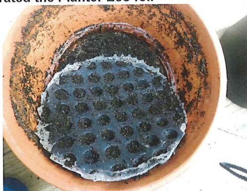
Photo No. 4 and 5 – The roots have not penetrated the Logicbase V-SL
